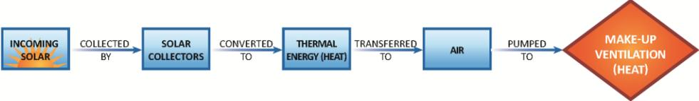
Figure 5. Flow Diagram of How a Solar Heated Air System Works
