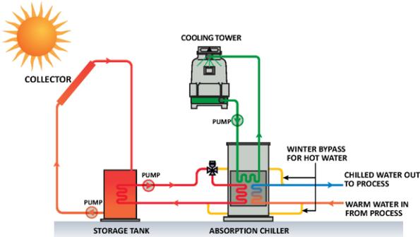
Figure 4. Drawing of a Solar Chilled Water System
