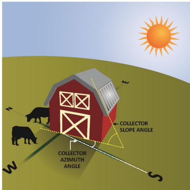
**Figure 7. Solar Collector Azimuth and Slope Angle**
