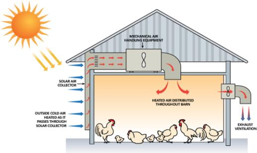
Figure 6. Drawing of a Solar Heated Air System
